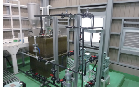
Delivery place : Kagoshima pref. Oil base Type : Powder polymer auto dissolver Model : PAD-Q20F-30
