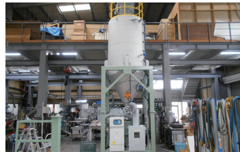
Delivery place : Wakayama pref. Final disposal site Type : Sodium carbonate auto dissolver Model : SAD-0.5S-5.0S
