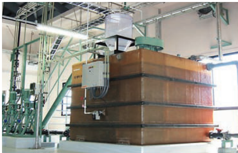
Delivery place : Tohoku region Waste disposal site Type : Powder polymer auto dissolver Model : PAD-D240F-250 (old model))
